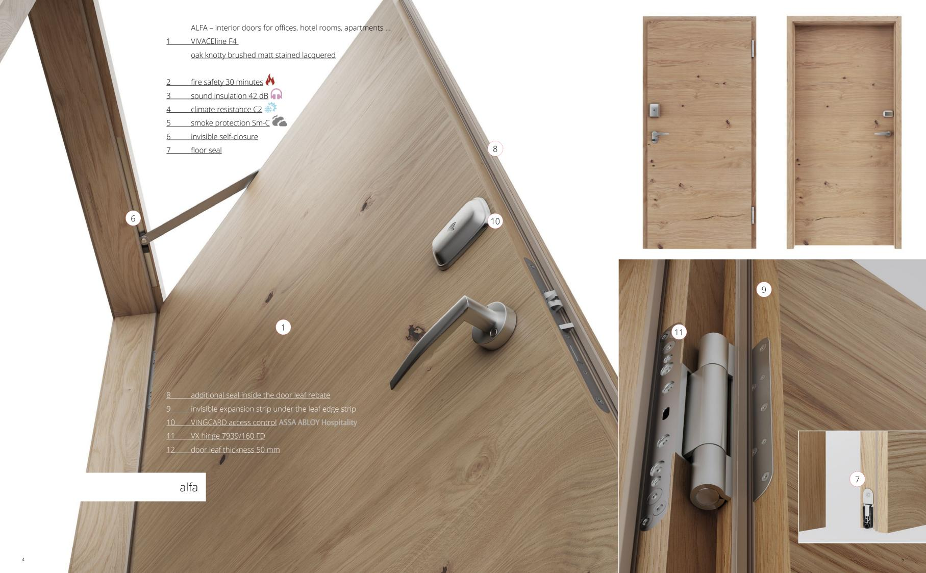
OMEGA – interior doors for offices, hotel rooms, apartments ... TOPline L1 oak knotty DYNAMIC cracked omega climate resistance C2 three-part hinges sound insulation 42 dB additional seal inside the door leaf rebate FORTE door leaf edges KFV three-point locking system door frame with rounded case profiles and rounded panel lining 5 floor seal
